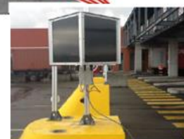
Automatic Gate-in inside the port area thanks to RFID antennas
